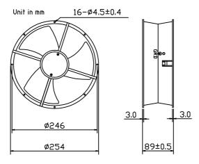
Housing: Aluminum painted black Impeller: PA6 Reinforced plastic(PBT) UL94V-0 Operating/working temperature: -10°C~60°C Lead Wire: 1015#20 AWG OR Equivalent Insulation Resistance:10M ohm,500VAC/min between bare and frame
