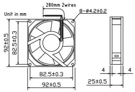
Housing: Aluminum Alloy painted black Impeller: PA6 Reinforced plastic(PBT) UL94V-0 Operating/working temperature: -10°C<sup>-</sup>60°C Lead Wire: 1007#22 AWG OR Equivalent Insulation Resistance:10M ohm,500VAC/min between bare and frame
