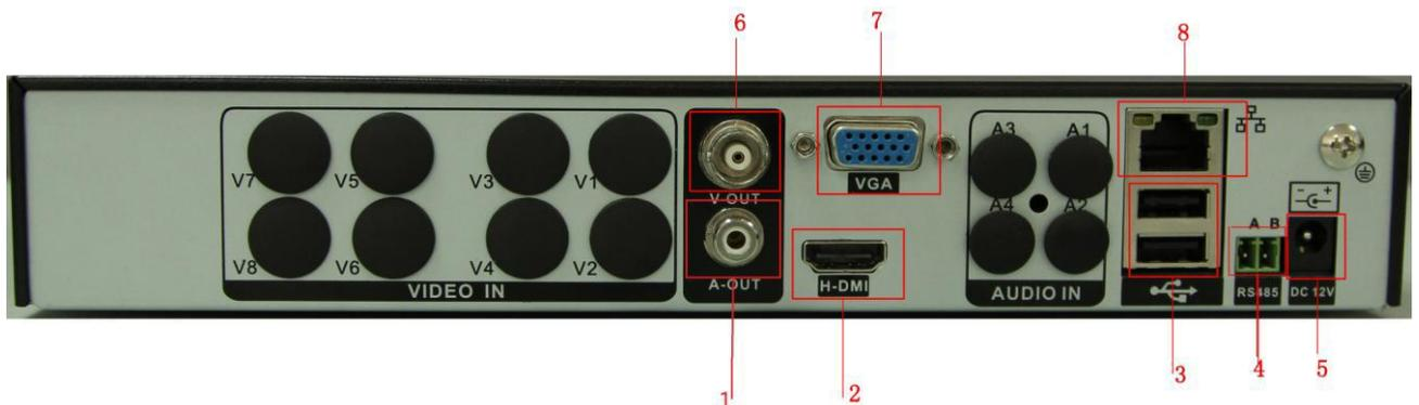
(1) Audio output (2)HDMI (3)USB (4)RS485 (5)Power (6)BNC (7)VGA (8)Network
