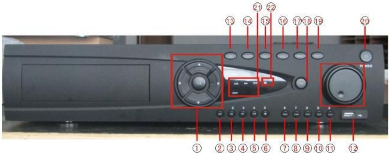
(1) Direction (2) Play Pause (3) Previous File (4) Next File (5) Backwards Pause (6) Play back Stop (7) Record check (8)Alarm output (9)Camera narrow (10) Camera zoom (11) Preset point set (12)USB (13)ESC (14) Scene switch (15)Record (16) PTZ (17)Menu (18)Assist (19)Shift (20) Power switch (21) Indicator light (22) IR remote receiver
