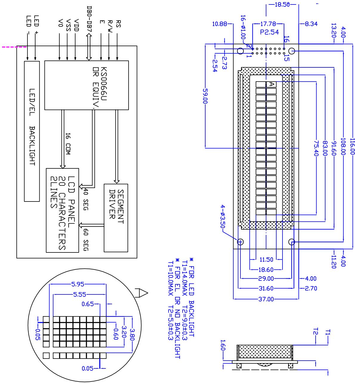
ALL DIMENSIONS ARE IN MM. TOLERANCE IS +/-0.2
