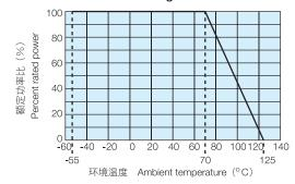
在环境温度70℃以上使用时,应按照上图负荷特性曲线,减小额定功率。 For resistors operated at an ambient temperature of 70℃ or above, a power rating shall be derated in accordance with the above derating curve.
