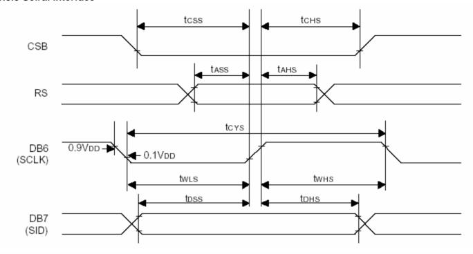
$(V_{DD} = 1.8V, Ta = -40 \text{ to } +85^{\circ}C)$
