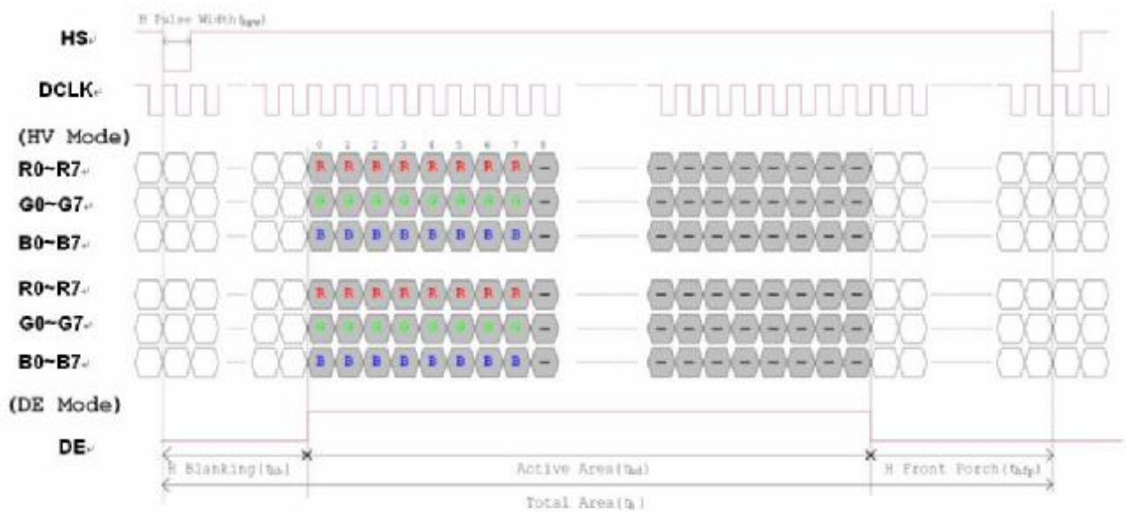
Figure 3. 1 Horizontal input timing diagram.
