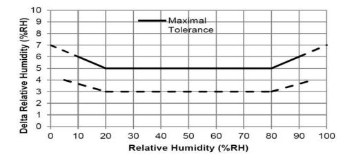
$\cdot$  The optimal measurement range specified by the HCH20DP sensor module is 5% RH—95% RH
